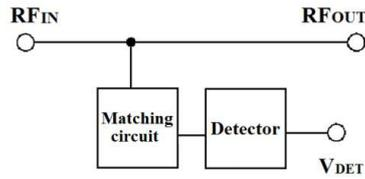
Fig. 13. Simplified circuit of non-directional detector
