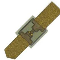
Fig. 1. Beam lead edition of ZB-28 diode
