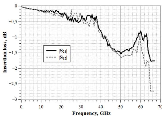
Fig. 16. MD908 insertion loss
