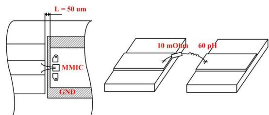
Fig. 7. MMIC connection with transmission line and bonding wires parameters
