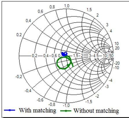
Fig. 8. The result of bonding wires matching
