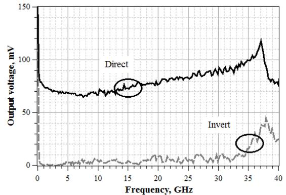
Fig. 12. Output voltage vs frequency for direct and invert modes at +10 dBm
