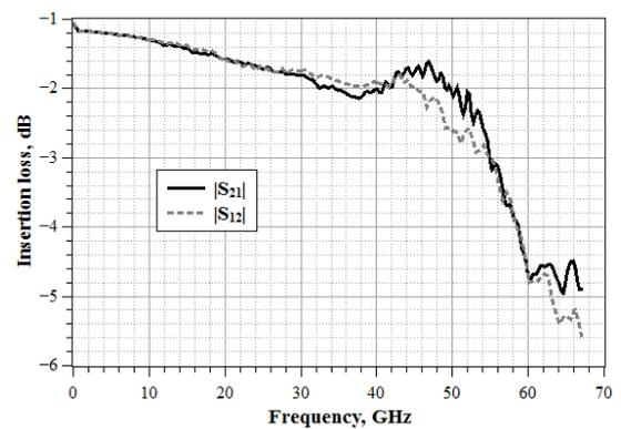
Fig. 6. MD902 insertion loss
