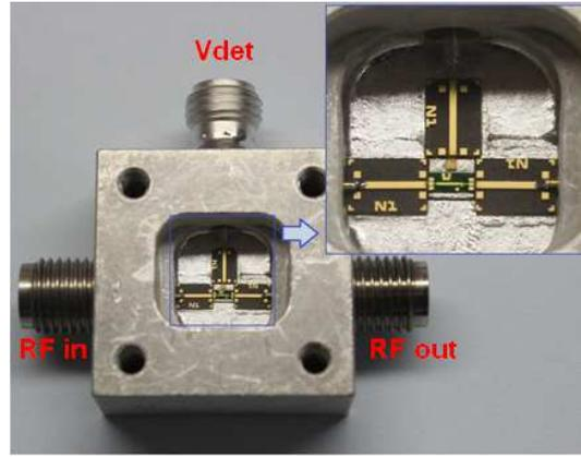
Fig. 11. Test RF module with MD902
