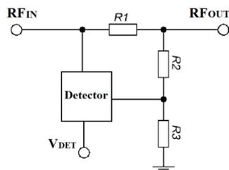
Fig. 3. Simplified circuit of the directional power detector
