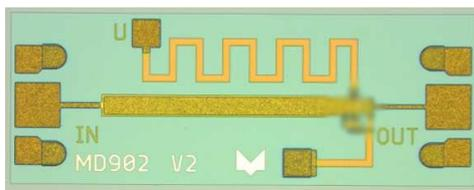
Fig. 4. MD902 directional power detector MMIC layout
