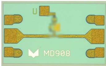
Fig. 14. MD908 non-directional power detector MMIC layout
