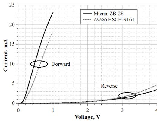
Fig. 2. IV-curves of zero bias diode
